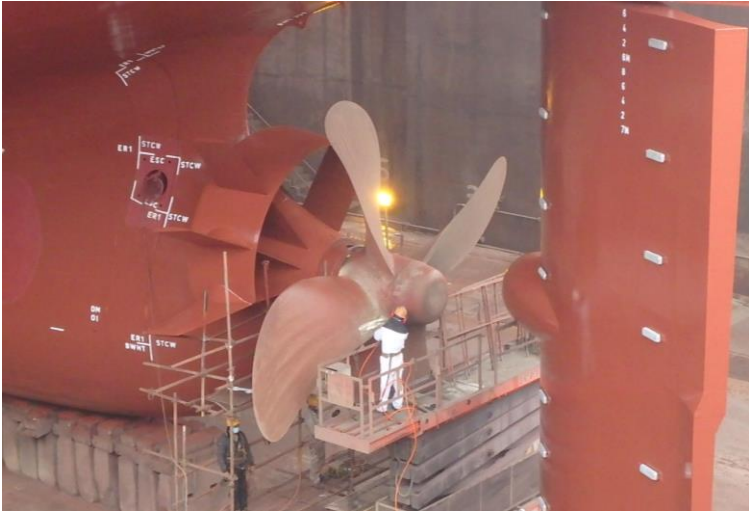
Installation of Becker-Mewis Duct aboard MV Baffin during dry dock
